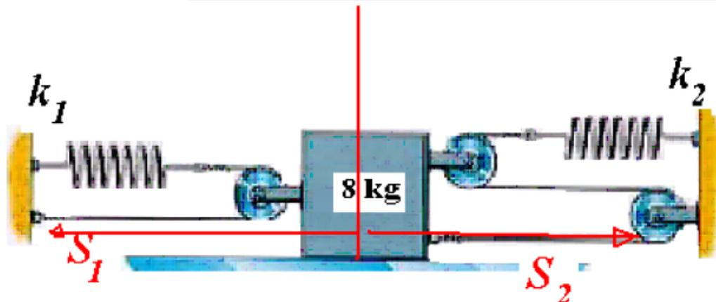
$$\left. \begin{aligned} 3T_2 - 2T_1 &= m\ddot{x} \\ T_1 &= k_1\delta_1(t) \\ T_2 &= k_2\delta_2(t) \end{aligned} \right\}$$
