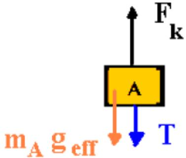
$$\left. \begin{aligned} F_k - T - m_A g_{eff} &= 0 \\ T - m_B g_{eff} &= 0 \end{aligned} \right\}$$
