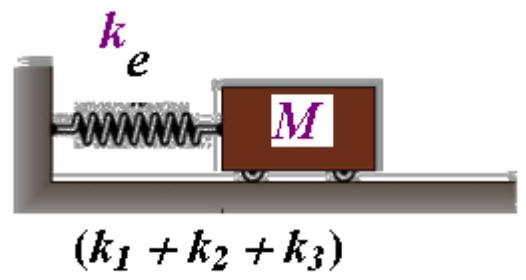
$$\omega_0 = \sqrt{\frac{(k_1 + k_2 + k_3)}{m}} \quad T = 2\pi \sqrt{\frac{(k_1 + k_2 + k_3)}{m}}$$
