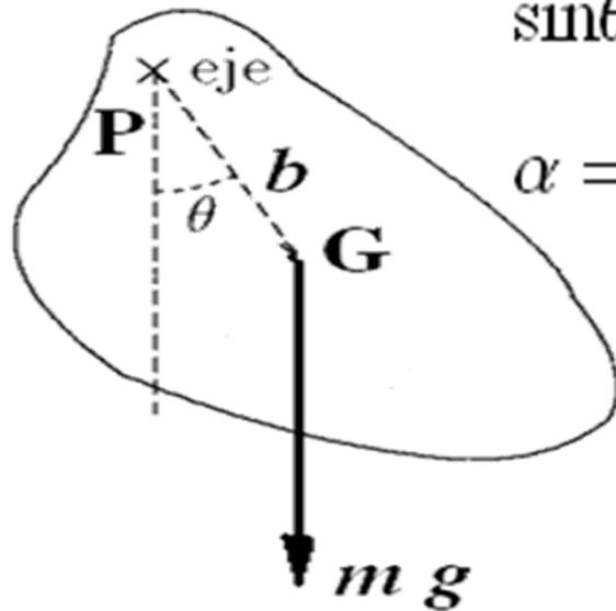
$$\sin\theta \simeq \theta \quad \vec{M}_P = \vec{PG} \wedge \vec{p} = -\sin\theta b m g \vec{k}$$
