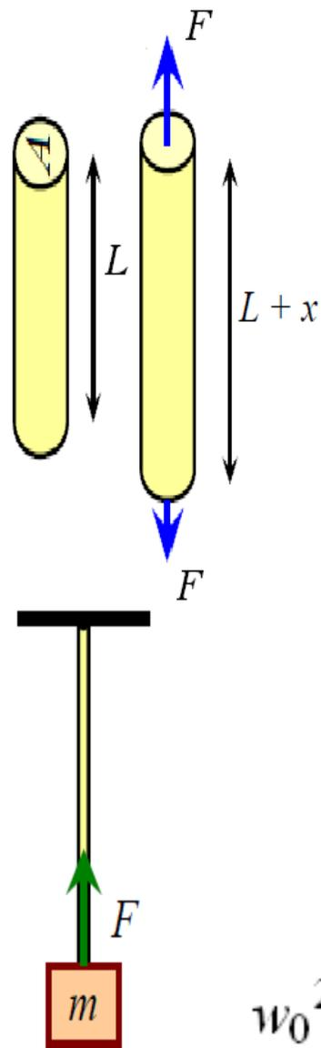
$$\left. \begin{aligned} \frac{F/A}{x/L} &= -Y \\ \frac{mL}{AY} &= \frac{x_e}{g} \\ \ddot{y} + \frac{gg}{x_e} y &= 0 \end{aligned} \right\} \Rightarrow \ddot{x} + \frac{k}{m} x = 0$$
