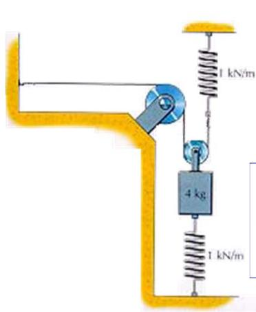
$$A = \frac{\sqrt{x_0^2 \omega_0^2 + v_0^2}}{\omega_0}$$
