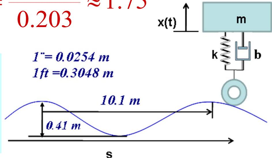
$$\frac{1}{\sqrt{\left(1 - \left(\frac{\omega}{\omega_0}\right)^2\right)^2 + \left(2\zeta \frac{\omega}{\omega_0}\right)^2}} = 1.75$$
