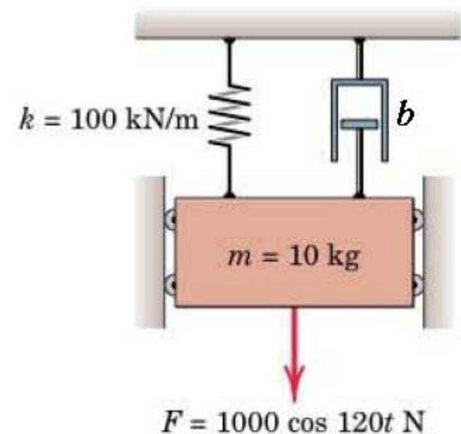
$$k \delta(t) + b v(t) - mg - F_0 \cos(\omega t + \alpha_0) = (-) m \ddot{y}(t)$$
