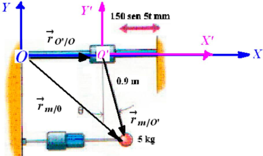
$$\vec{r}_{m/O} = \vec{r}_{m/O'} + \vec{r}_{O'/O} = l(\sin \theta, -\cos \theta) + (z_0 \sin \Omega t, 0) = (l \sin \theta + z_0 \sin \Omega t, -l \cos \theta)$$
