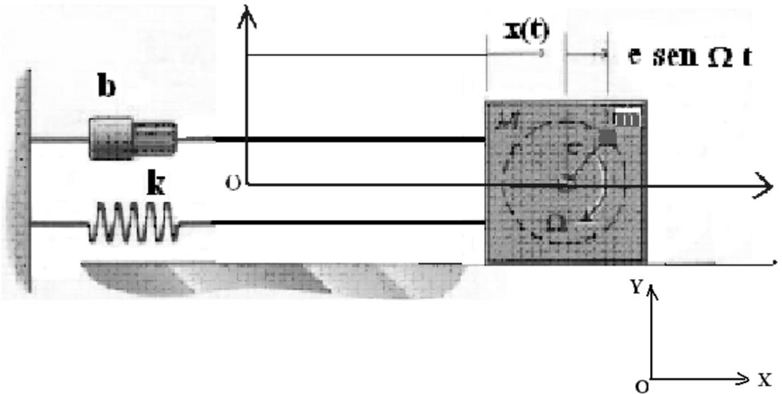
$$\vec{x}_{CM}(t) = (x_{CM}, y_{CM}) = \frac{m_1 \vec{x}_1(t) + m_2 \vec{x}_2(t)}{m_1 + m_2} = \frac{M(x(t), 0) + m(x(t) + x_m(t), y_m(t))}{M + m}$$
