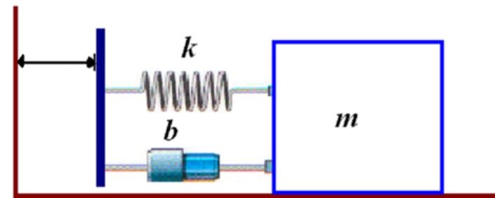
$$z_p(t) = z_0 \sin \Omega t \text{ mm}$$
