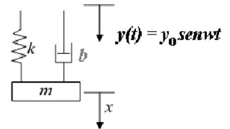
$$\ddot{x} + \frac{b}{m} \dot{x} + \frac{k}{m} x = \sqrt{\left(\frac{k y_0}{m}\right)^2 + \left(\frac{b \omega}{m} y_0\right)^2} \text{Sen} \left(\omega t + \tan^{-1} \left(\frac{b \omega}{k}\right)\right)$$
