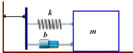
$$\ddot{x} + 2\gamma \dot{x} + \omega_0^2 x = g_0 \text{Cos}(\Omega t + \alpha_0)$$
