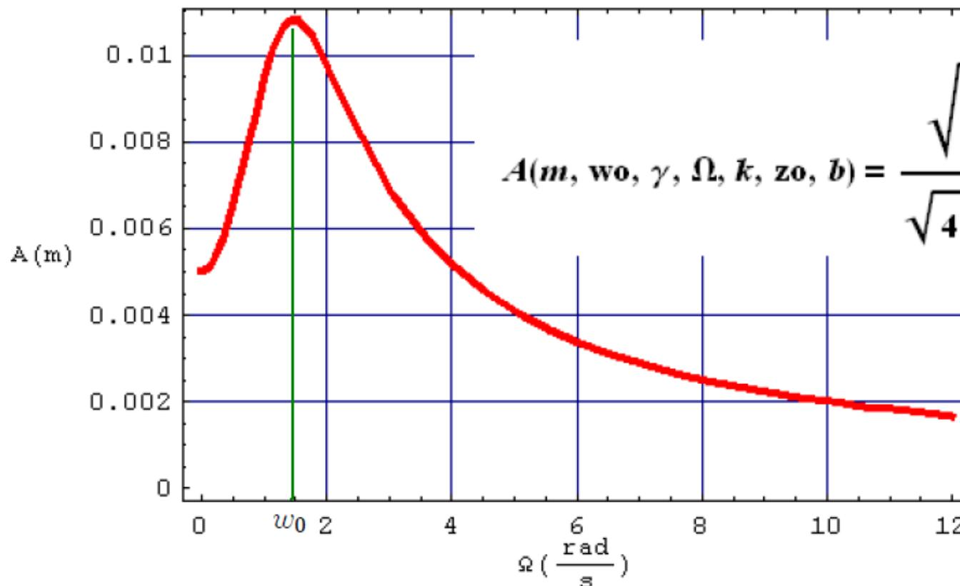
$$A(m, \omega_0, \gamma, \Omega, k, z_0, b) = \frac{\sqrt{\left(\frac{k z_0}{m}\right)^2 + \left(\frac{b z_0 \Omega}{m}\right)^2}}{\sqrt{4 \gamma^2 \Omega^2 + (\omega_0^2 - \Omega^2)^2}}$$
