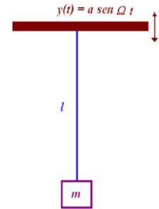
$$\delta(t) = \delta_e - a \operatorname{sen}(\Omega t) \left( -1 + \frac{1}{\sqrt{\left(1 - \left(\frac{\Omega}{\sqrt{\frac{g}{\delta_e}}}\right)^2\right)^2}} \right) \geq 0 \quad \Rightarrow \quad a \leq \frac{\delta_e}{\left( \frac{1}{\sqrt{\left(1 - \left(\frac{\Omega}{\sqrt{\frac{g}{\delta_e}}}\right)^2\right)^2}} - 1 \right)}$$
