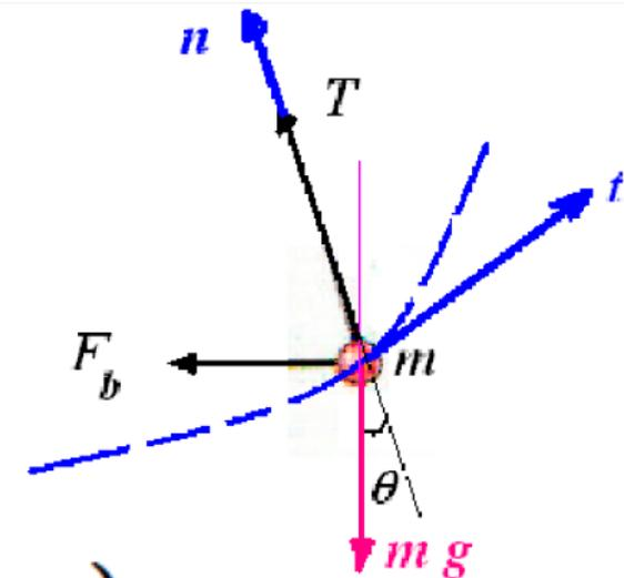
$$\left. \begin{aligned} -mg \sin \theta - F_b \cos \theta &= ma_t = m \frac{dv}{dt} \\ T - mg \cos \theta + F_b \sin \theta &= m a_n = m \frac{v^2}{L} \end{aligned} \right\} \Rightarrow \frac{dv}{dt} = \frac{d}{dt} (z_0 \Omega \cos(\Omega t) + l\dot{\theta}) = -z_0 \Omega^2 \sin \Omega t + l\ddot{\theta}$$
