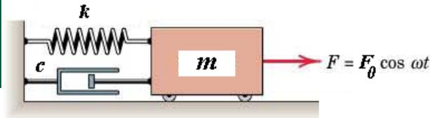
$$\omega_0 = +\sqrt{\frac{k}{m}} = +\sqrt{\frac{1051}{286.6/9.81}} = 6 \frac{\text{rad}}{\text{s}} \quad \zeta = 0$$
