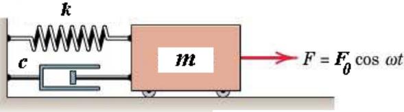
$$\frac{A}{\left(\frac{g_0}{\omega_0^2}\right)} = \frac{1}{\left(1 - \left(\frac{\omega}{\omega_0}\right)^2\right)} \frac{g_0}{\omega_0^2} = \frac{\frac{F_0}{m}}{\omega_0^2} = \frac{F_0}{m \omega_0^2} = \frac{22.24}{(286.6/9.81)^2} = 0.021 \text{ m}$$
