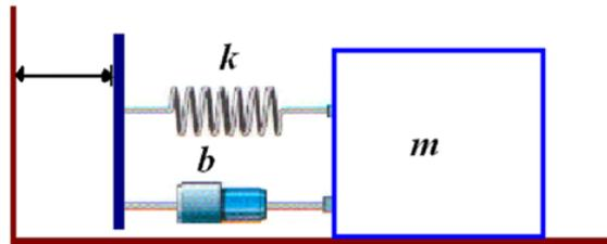
$$\ddot{x} + \frac{k}{m} x + \frac{b}{m} \dot{x} = \frac{k}{m} z_0 \sin \Omega t + \frac{b}{m} z_0 \Omega \cos \Omega t$$
