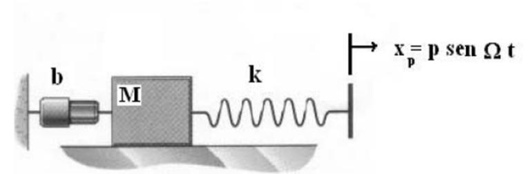
$$\ddot{x}(t) + 2\gamma \dot{x}(t) + \omega_0^2 x(t) = k p \text{ sen } \Omega t$$
