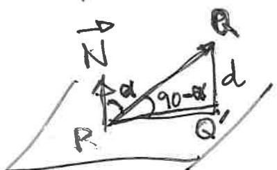
$$\begin{aligned} d &= |\vec{PQ}| \sin(90^\circ - \alpha) = |\vec{PQ}| \cos \alpha \\ &= |\vec{PQ}| |\vec{N}| \cos \alpha = |\vec{PQ}| |\vec{N}| \cos \alpha \\ &= \vec{PQ} \cdot \vec{N} \end{aligned}$$
